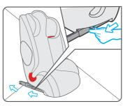
Push the ISOFIX connectors directly into the anchorages until heard an audible sound.
