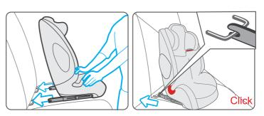
Grasp the seat body to check the seat if it is fastened tightly or shakes. if the seat shakes and the ISOFIX connectors are pulled out, please repeat the above steps and install it.
