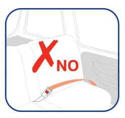
**NOTE:** that the seat is only suitable for fitting on a car seat compliant with ECE R16 or equivalent standards with a three-point seat belt with an emergency locking retractor.
